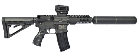
The Truvelo TM 545P-SF is a 5.56x45mm adjustable piston operated rifle. Both the upper and lower receiver are made from precision forged 7075-T6 Aluminium, with the upper receiver benefiting from an extended M4 feed ramp. The 12" cold forged rifled barrel is made from high alloy Chrome Molybdenum steel with a final Nitride Treatment for strength and endurance.
