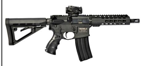
The TM 545 CQR is a 5.56x45mm direct impinged gas operated rifle. Both the upper and lower receiver are from precision forged 7075-T6 Aluminium, with the upper receiver benefiting from an extended M4 feed ramp. The 10" cold forged rifled barrel is made from high alloy Chrome Molybdenum steel with a final Nitride Treatment for strength and endurance.
