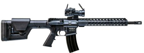
The TM 545 DMR is a 5.56x45mm direct impinged gas operated Precision rifle. Both the upper and lower receiver are from precision forged 7075-T6 Aluminium, with the upper receiver benefiting from an extended M4 feed ramp. The 16" cold forged rifled barrel is made from high alloy Chrome Molybdenum steel with a final Nitride Treatment for strength and endurance. The Truvelo TM 545 DMR comes standard with the Magpul PRS Gen 3 Stock.
