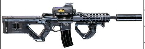
The TM 545 CQR - XS is a 5.56x45mm direct impinged gas operated rifle. Both the upper and lower receiver are from precision forged 7075-T6 Aluminium, with the upper receiver benefiting from an extended M4 feed ramp. The 9" cold forged rifled barrel is made from high alloy Chrome Molybdenum steel with a final Nitride Treatment for strength and endurance. Furniture include the Hera CQR Stock and fore-end.
