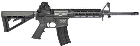
The TM 545 Commando is a 5.56x45mm direct impinged gas operated rifle. Both the upper and lower receiver are from precision forged 7075-T6 Aluminium, with the upper receiver benefiting from an extended M4 feed ramp. The 12" cold forged rifled barrel is made from high alloy Chrome Molybdenum steel with a final Nitride Treatment for strength and endurance. Variety of furniture options available.
