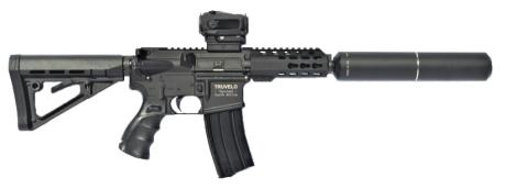
The TM-300 BLK is a 7.62x35mm direct impinged gas operated rifle. Both the upper and lower receiver are made from precision forged 7075-T6 Aluminium, with the upper receiver benefiting from an extended M4 feed ramp. The 12" cold forged rifled barrel is made from high alloy Chrome Molybdenum steel with a final Nitride Treatment for strength and endurance.
