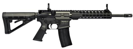
The TM 545 Carbine is a 5.56x45mm direct impinged gas operated rifle. Both the upper and lower receiver are from precision forged 7075-T6 Aluminium, with the upper receiver benefiting from an extended M4 feed ramp. The 14.5" cold forged rifled barrel is made from high alloy Chrome Molybdenum steel with a final Nitride Treatment for strength and endurance. Variety of furniture options available.
