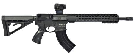
The Truvelo TM 739 Special Operations is a 7,62x39mm direct impinged gas operated rifle. Both the upper and lower receiver are made from precision forged 7075-T6 Aluminium, with the upper receiver benefiting from an extended M4 feed ramp. The 12" cold forged rifled barrel is made from high alloy Chrome Molybdenum steel with a final Nitride Treatment for strength and endurance.
