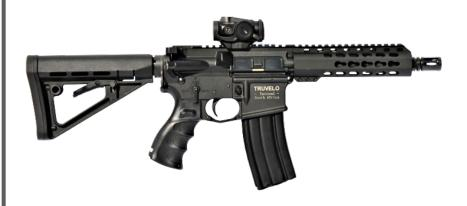
The TM 545 CQR is a 5.56x45mm direct impinged gas operated rifle. Both the upper and lower receiver are made from precision forged 7075-T6 Aluminium, with the upper receiver benefiting from an extended M4 feed ramp. The 9" cold forged rifled barrel is made from high alloy Chrome Molybdenum steel with a final Nitride Treatment for strength and endurance.
